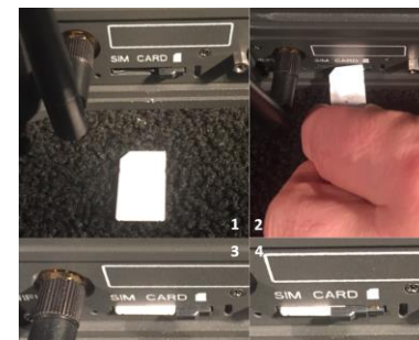
Installing SIM card and engaging the lock
